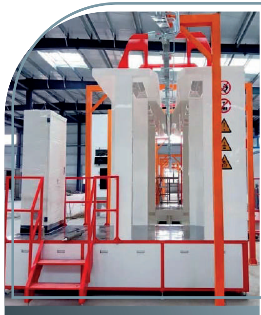
AUTOMATIC POWDER COATING LINE WITH NANO TECHNOLOGY
